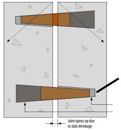
As the panels shrink, a small void is formed in the concrete by the tapered shape of the plate dowels, thereby minimising restraint induced stresses.
